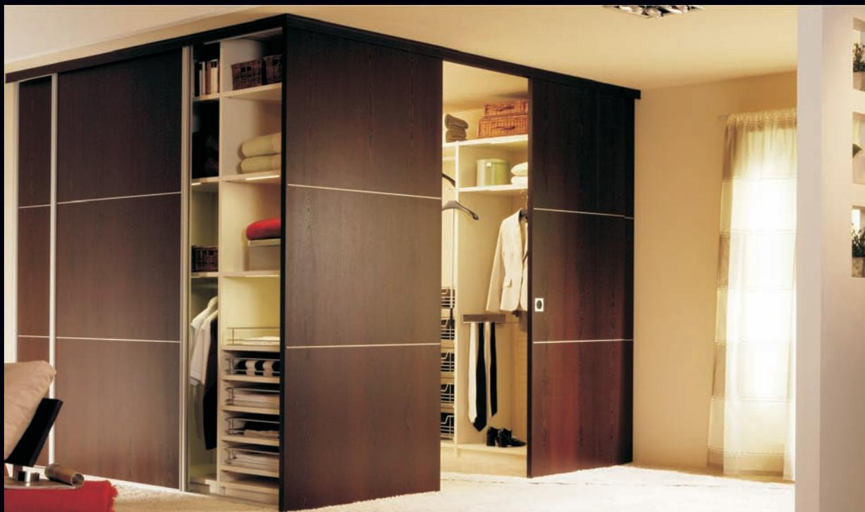
**All-wood** system is based on sliding doors which main advantage is space economy and functionality. **All-wood** system is used in various solutions (built-in closets, partition systems, delimitation constructions). **All-wood** is equipped with roller mechanism door. Minimum covering of the doors is 30 mm. **All-wood** maximal door leaf width is **1200 mm**, maximal door height – **2590 mm**.
